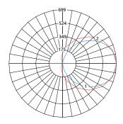
Max Candela = 699 Located At Horizontal Angle = 0, Vertical Angle = 90 1 - Vertical Plane Through Horizontal Angles (0-180) (Through Max. Cd.) 2 - Horizontal Cone Through Vertical Angle (90) (Through Max. Cd.)
