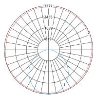
Maximum Candela = 3277 Located At Horizontal Angle = 15, Vertical Angle = 5
