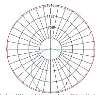
$Maximum\ Candela = 1516\ Located\ At\ Horizontal\ Angle = 15, Vertical\ Angle = 5$
