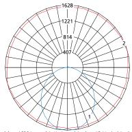
Maximum Candela = 1628 Located At Horizontal Angle = 15, Vertical Angle = 5
