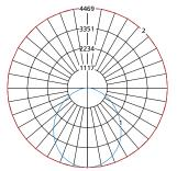
Max Candela = 4469 Located At Horizontal Angle = 0, Vertical Angle = 0
