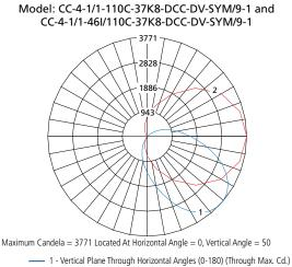
— 2 - Horizontal Cone Through Vertical Angle (50) (Through Max. Cd.)
