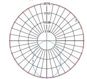
Maximum Candela = 2076 Located At Horizontal Angle = 15, Vertical Angle = 2.5
