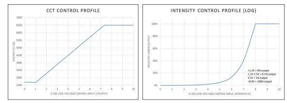
NOTE: The provided information is the typical expected performance of a single luminaire. Additional luminaires on the same 0-10V line may result in different control profiles. Fine tuning of system performance should be completed after installation is complete. To avoid CCT shift between luminaires, care should be taken to minimize voltage drop on the CCT Control line. It is recommended to limit the load on the CCT control circuit to twenty (20) luminaires or less.
