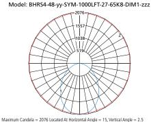
1 - Vertical Plane Through Horizontal Angles (15-195) (Through Max. Cd.)
