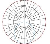
Maximum Candela = 3809 Located At Horizontal Angle = 0, Vertical Angle = 0
