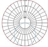
Maximum Candela = 1520 Located At Horizontal Angle = 0, Vertical Angle = 0 1 - Vertical Plane Through Horizontal Angles (0-180) (Through Max. Cd.)
