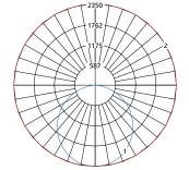
Maximum Candela = 2350 Located At Horizontal Angle = 0, Vertical Angle = 0 1 - Vertical Plane Through Horizontal Angles (0-180) (Through Max. Cd.)
