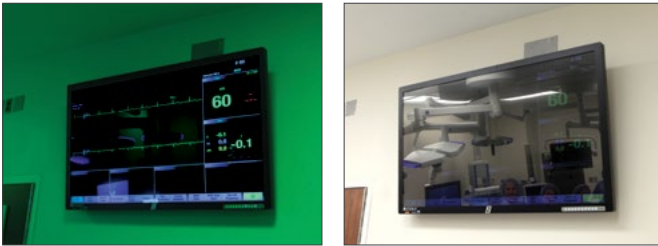
530nm "green" LED light significantly reduces monitor glare to allow the medical staff to see clearly without adjusting the lights.
