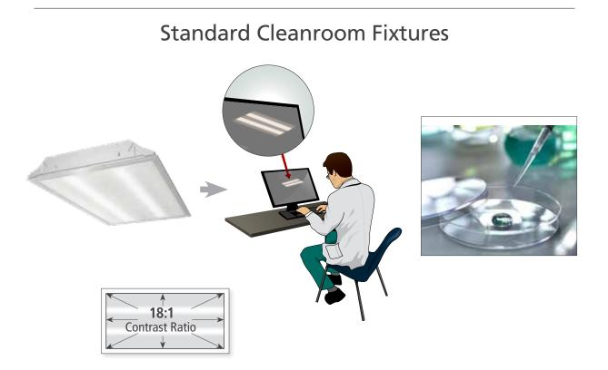
**Competitor Fixtures:** Fixtures that use linear LED boards and prismatic-pattern lenses create very high contrast – as high as an 18:1 max. to min. ratio.
