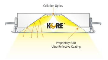
The CSERO/CSERI luminaires feature Kenall's patent-pending KORE (Kenall Optical Radiance Engine) Technology<sup>™</sup>, which dramatically increases efficacy and eliminates debilitating glare.
