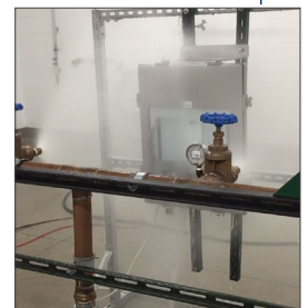
Water Ingress Testing
