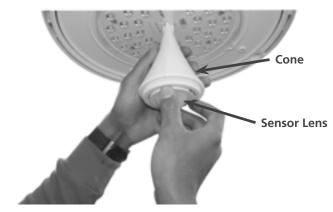
3. Adjust sensor to desired time, Mode and Dim Level (see page 4)
