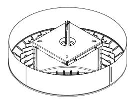
2. Bird Guard lays inside of casting.
