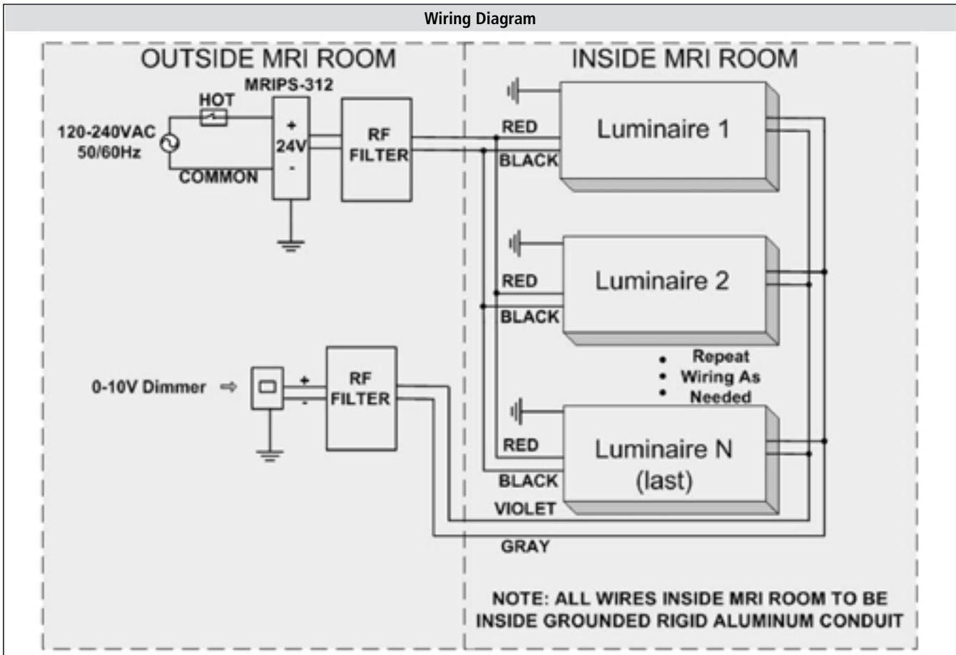
12. Run the 24VDC supply from the EMI filter to the luminaire(s) using at least 18 AWG wires. Class 1 wiring is required. Make sure wiring is completely enclosed in grounded aluminum conduit. Any gaps, regardless of size, must be closed or wrapped in copper foil tape. Special attention should be paid to the wiring entry point into the shielded space. See Figure above.
