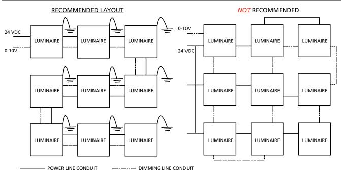
Multi-Fixture System Schematic
