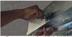
3. Remove four (4) 1/4 turn screws and remove electrical tray.
