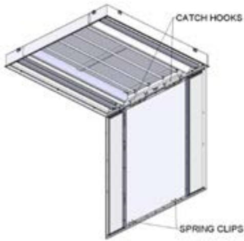
Figure 1 - Internal Door Hinge
