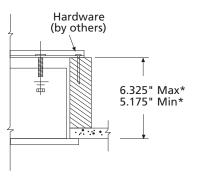
Mounting method when fixture is supported in a wood frame construction.
