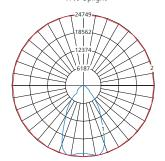
Max Candela = 24749 Located At Horiz. Angle = 75, Vertical Angle = 12.5 1 - Vertical Plane Through Horiz. Angles (75-255) (Through Max. Cd.) 2 - Horizontal Cone Through Vert. Angle (12.5) (Through Max. Cd.) Model: EPHB-16-U1-PM-CP-GW-224L-40K8-DCC-DV 8% Uplight
