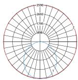
$Maximum\ Candela = 3590\ Located\ At\ Horizontal\ Angle = 15,\ Vertical\ Angle = 5$
