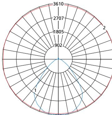
Maximum Candela = 3610 Located At Horizontal Angle = 15, Vertical Angle = 5
