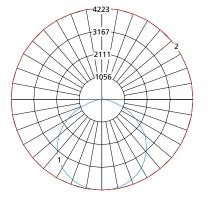
Maximum Candela = 4223 Located At Horizontal Angle = 210, Vertical Angle = 5
