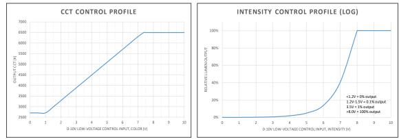
NOTE: The provided information is the typical expected performance of a single luminaire. Additional luminaires on the same 0-10V line may result in different control profiles. Fine tuning of system performance should be completed after installation is complete. To avoid CCT shift between luminaires, care should be taken to minimize voltage drop on the CCT Control line. It is recommended to limit the load on the CCT control circuit to twenty (20) 45T or ten (10) 67T/90T luminaires or less.
