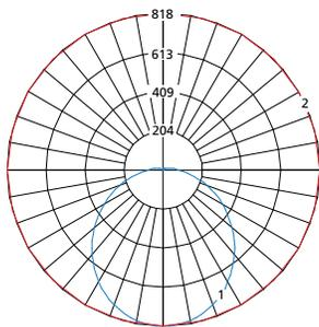
Max Candela = 818 Located At Horizontal Angle = 0, Vertical Angle = 0
