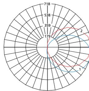
Max Candela = 718 Located At Horizontal Angle = 0, Vertical Angle = 65
