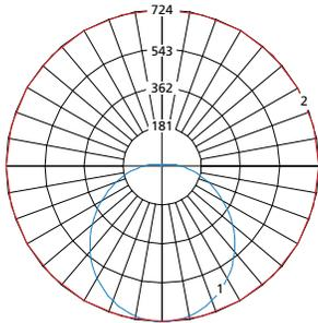
Max Candela = 724 Located At Horizontal Angle = 0, Vertical Angle = 0
