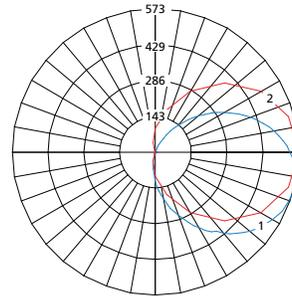
Max Candela = 573 Located At Horizontal Angle = 0, Vertical Angle = 65
