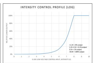
NOTE: The provided information is the typical expected performance of a single luminaire. Additional luminaires on the same 0-10V line may result in different control profiles. Fine tuning of system performance should be completed after installation is complete. To avoid CCT shift between luminaires, care should be taken to minimize voltage drop on the CCT Control line. It is recommended to limit the load on the CCT control circuit to twenty (20) 45T or ten (10) 67T/90T luminaires or less.
