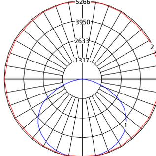
Max Candela = 5266 Located At Horizontal Angle = 45, Vertical Angle = 42.5
