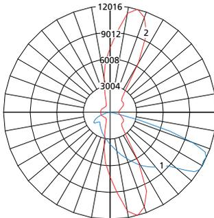
Max Candela = 12016 Located At Horizontal Angle = 75, Vertical Angle = 57.5
