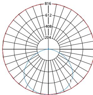
Max Candela = 816 Located At Horizontal Angle = 0, Vertical Angle = 0
