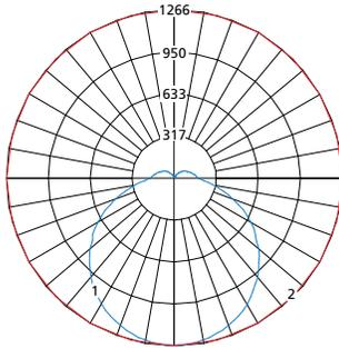
Max Candela = 650 Located At Horizontal Angle = 0, Vertical Angle = 75
