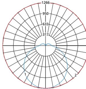
Max Candela = 1266 Located At Horizontal Angle = 0, Vertical Angle = 0
