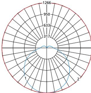
Max Candela = 650 Located At Horizontal Angle = 0, Vertical Angle = 75
