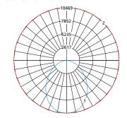
$\label{eq:max-candel} \mbox{Max Candela} = \mbox{10469 Located At Horizontal Angle} = \mbox{0, Vertical Angle} = \mbox{0}$
