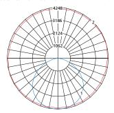
$\label{eq:maximum Candela} {\sf Maximum Candela} = 4248 \ {\sf Located At Horizontal Angle} = 15, {\sf Vertical Angle} = 5$
