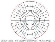
1 - Vertical Plane Through Horizontal Angles (195-15) (Through Max. Cd.)
