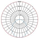
Max Candela = 4560 Located At Horizontal Angle = 0, Vertical Angle = 0 1 - Vertical Plane Through Horizontal Angles (0 - 180) (Through Max. Cd.) 2 - Horizontal Cone Through Vertical Angle (0) (Through Max. Cd.)
