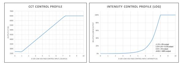
NOTE: The provided information is the typical expected performance of a single luminaire. Additional luminaires on the same 0-10V line may result in different control profiles. Fine tuning of system performance should be completed after installation is complete. To avoid CCT shift between luminaires, care should be taken to minimize voltage drop on the CCT Control line. It is recommended to limit the load on the CCT control circuit to twenty (20) 45T or ten (10) 67T/90T luminaires or less.
