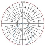
Max Candela = 4304 Located At Horizontal Angle = 0, Vertical Angle = 0 1 - Vertical Plane Through Horizontal Angles (0 - 180) (Through Max. Cd.) 2 - Horizontal Cone Through Vertical Angle (0) (Through Max. Cd.)
