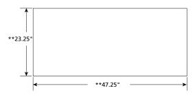
\*\* Add .25" to each cut-out dimension when Install Frame (IF) accessory is specified.
