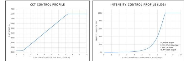
NOTE: The provided information is the typical expected performance of a single luminaire. Additional luminaires on the same 0-10V line may result in different control profiles. Fine tuning of system performance should be completed after installation is complete. To avoid CCT shift between luminaires, care should be taken to minimize voltage drop on the CCT Control line. It is recommended to limit the load on the CCT control circuit to twenty (20) 45T or ten (10) 67T/90T luminaires or less.
