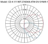
Maximum Candela = 4275 Located At Horizontal Angle = 0, Vertical Angle = 45
