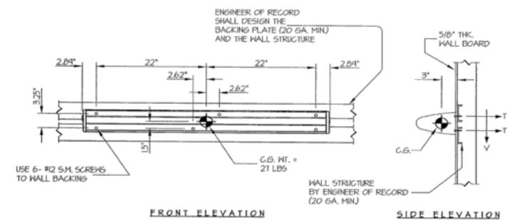
LOADS: PER 2007 CALIFORNIA BUILDING CODE SECTION 1613A AND ASCE 7-05 SECTIONS 12 AND 13. WEIGHT = 27 LBS HORIZONTAL FORCE (Eh) = 0.70 Wp = 19 LBS VERTICAL FORCE (Ev) = 0.19 Wo = 5 LBS
