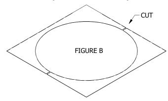
3. Place fixture in t-grid ceiling without tile. Use swingout arms to rest on t-grid.
