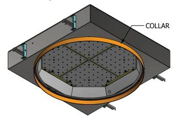
4. Fixture collar to be adjusted flush with the bottom of ceiling tile. Use adjustment screw to raise or lower fixture.
