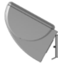
5. Hook luminaire onto wall plate tabs.
