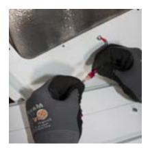
16. Secure Electrical assembly to Top Base with (4) captive screw provided.
